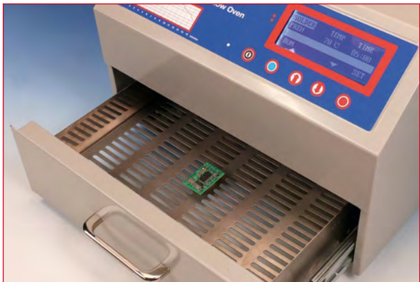
Figure 6. Our first 'guinea pig' is ready to face the IR heat in our reflow oven.
