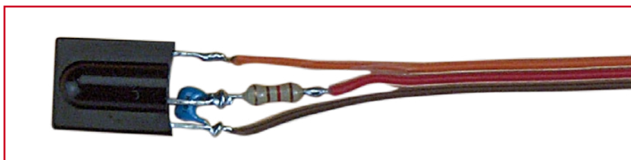
Figure 5. TSOP with RC (resistor-capacitor) filter and connecting wires.
