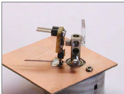
The complete servo including the magnet sensor which is held in the correct place with a small PCB.
