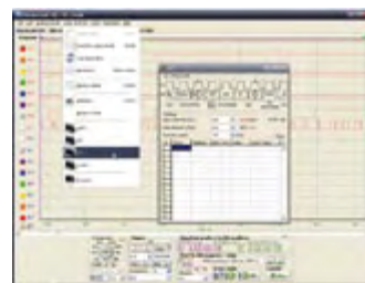
UART, SPI, I2C and 1-wire decoding view
