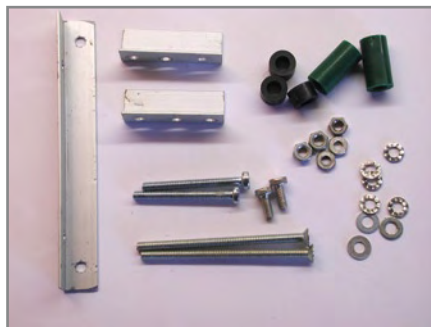
We make the mechanical construction with M3 hardware and aluminium angle profile.
