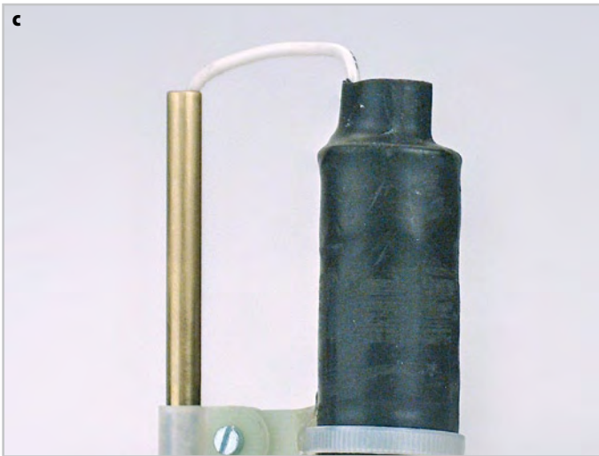
Figure 5. Details of the prototype assembly: (a) base plate (aluminium heat sink), (b) Hall sensor, (c) brass rod with coil leads, (d) coil bracket with cable ties.
