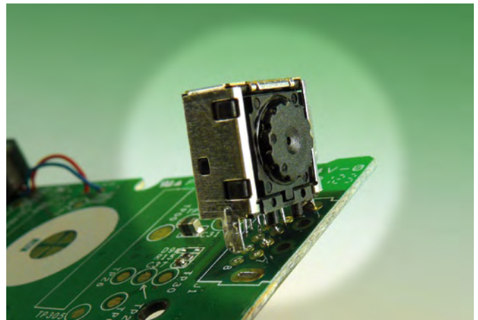
Figure 6. The solder tabs of the sheet-metal screen are a bit more stubborn.
