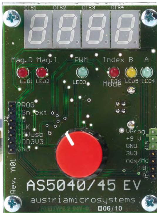
Figure 6. An AS50xx demonstration board provides a development environment for dedicated applications using its accompanying free software.
